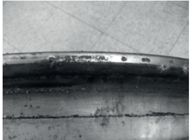
Picture 13-38 Acceptable pitting
