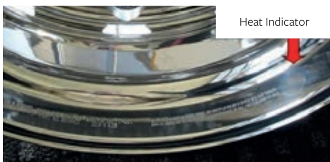
Picture 13-4 Heat indicator version 2
