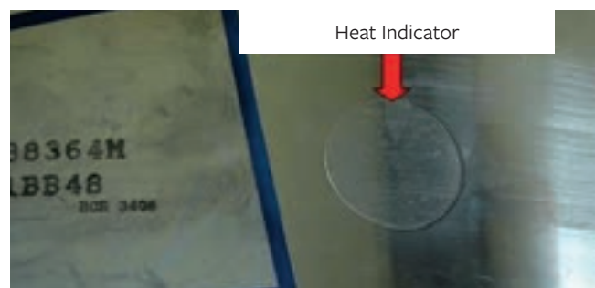
Picture 13-5 Heat indicator version 2 at wheel drop well, close to serial number and valve hole
